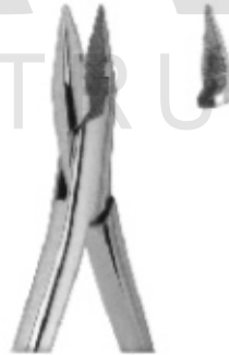
3216 Universal Universal pin roughening, cutting and bending pliers. For wires up to 0,9 mm. (.035"). Will cut wires up to 0,7 mm. (.028").
